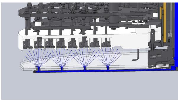
The automatic caps washing system (controlled via HMI) is integrated into Spiral Buffer device, so an operator to clean base disc with waterhose is not necessary anymore
