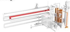
Option 2: New solution with shell and tube heat exchanger
